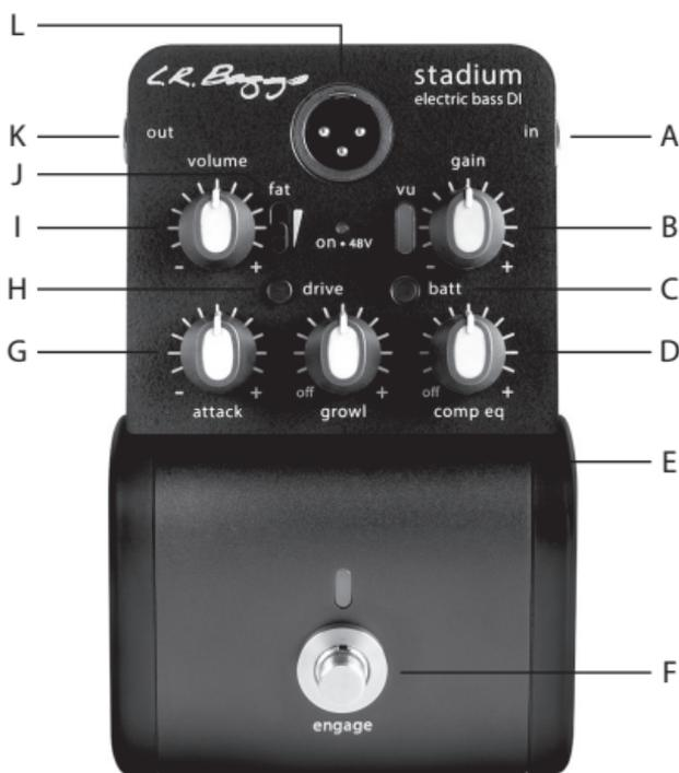
gain control in the counter-clockwise position. Turn the control clockwise as you play until the VU meter flashes yellow consistently. If red flashes too frequently, the input is clipping and you may experience unwanted distortion.
