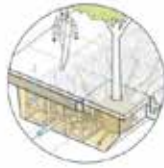
Use of soil cells or structural soils for new trees in paved areas
