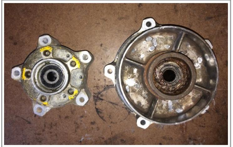
2. Then we will blast the hubs to remove the old paint and corrosion. We normally leave the old bearings in place at this stage to protect the machined housing.
