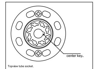
Some tubes and tube sockets have a "center key" which must line up! If you misalign them and use brute force, you will damage important and expensive parts of your amplifier!!
