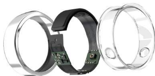
Figure 15. The Oura Ring, which stages sleep using pulse and temperature. Image from Ouraring.com.
