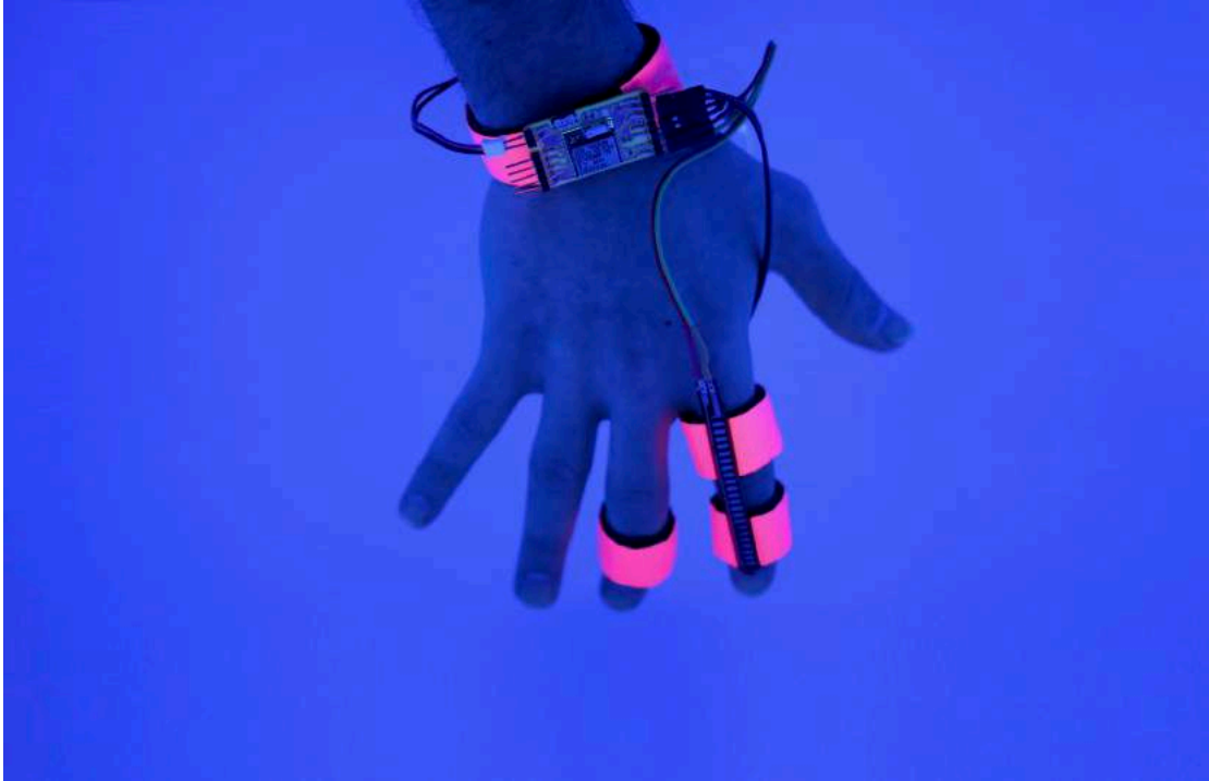
Figure 21. The Dormio PCB and handworn system, dorsal side. Photo credit Oscar Rosello
