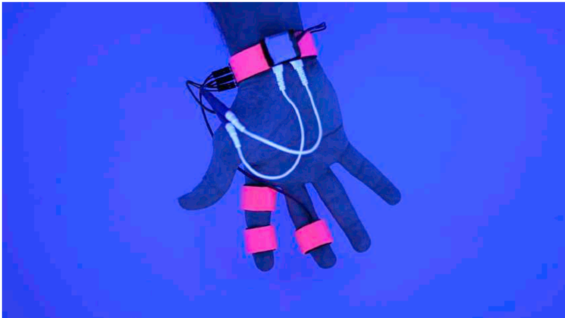
Figure 22. The Dormio PCB and handworn system, palmar side. Photo credit Oscar Rosello
