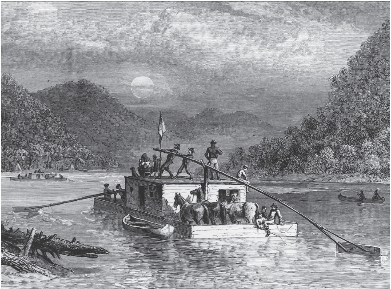
A group of people along with horses on board a flatboat, as they travel down a river under a moonlit sky. The flatboat was a creation of the Ohio River valley and moved downstream only. It was generally steered behind the stern, with a long swing oar as long as the boat itself, and by two "sweeps" forward, one on each side. Going down the Alleghany River, the Gooch family had, as their crew, a pilot, a steerman, and two men on the oars. Note the skiff tied to the side of the oar and the Indian canoe at the right. Engraving by Alfred A. Waud. Courtesy of The New York Public Library.
