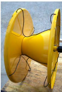
Tie wires bent to shape of cone
