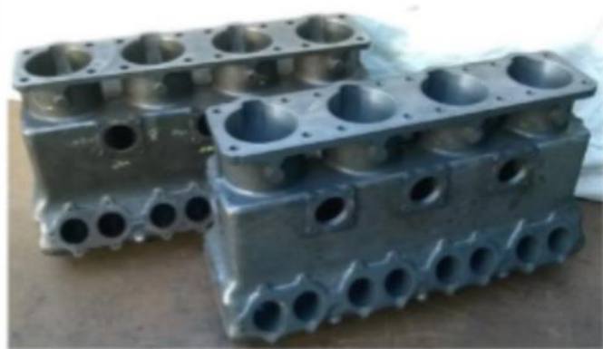
Production casting partly machined (with original).
