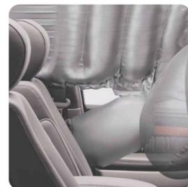
The Lexus LX's standard airbag configuration consists of **front seat-mounted side airbags**, **Roll-Sensing Curtain Airbags**, and driver and front-passenger airbags. The airbags are **Supplemental Restraint Systems (SRS)**
