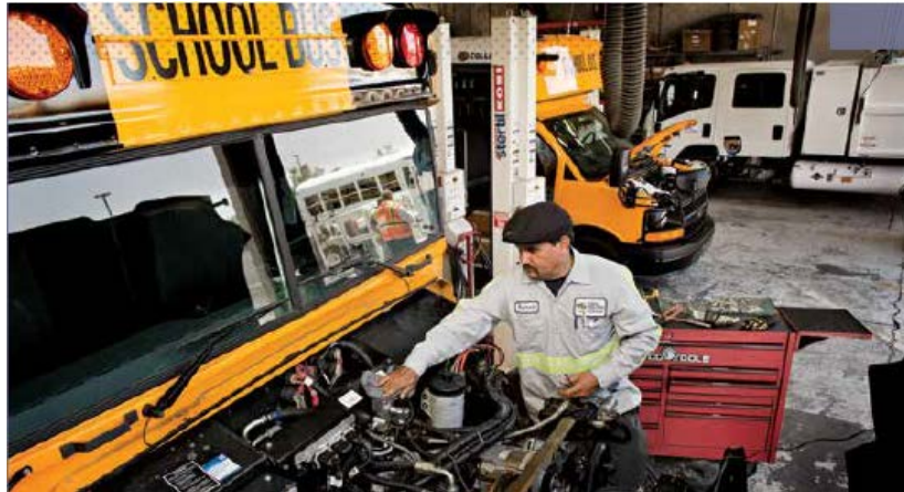
Figure 7: Maintenance on NGVs and propane autogas vehicles is similar to gasoline and diesel vehicles. Maintenance costs are also similar or even less, depending on specific duty cycle and engine platform.
