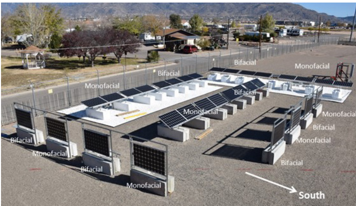
Figure 11. Module-scale bifacial PV test bed at Sandia National Laboratories Source: Sandia National Laboratories
