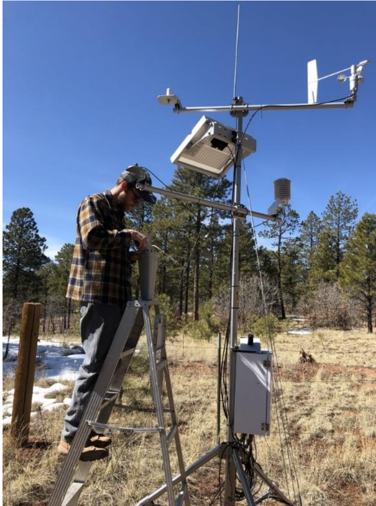
Photo 2: Sam Berry with The Forest Stewards Guild installs new antenna on the RAWS
