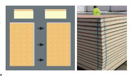
creates the recommended APA spacing. See illustration for guidance on orientation of boards. When cutting is necessary, make cuts on flush edges. Before packaging, the bundle is marked down the edge to designate the corner where adjacent sides contain non-flush edges. **NOTE: Due to variations in wood dimensions and tolerances, as well as, uncontrollable ambient conditions that can alter wood dimensions at the time of installation, the proper overhang is not always present.**
