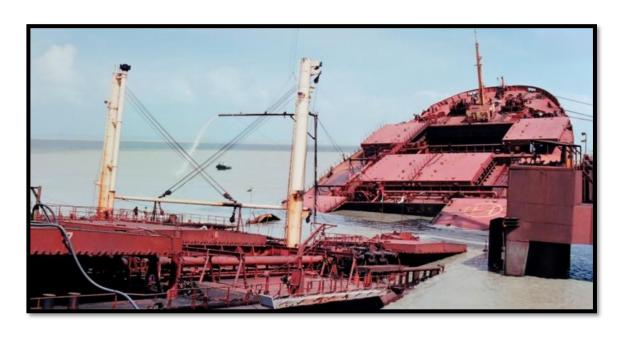
Hull Stress Monitoring Systems are present to prevent misloading
