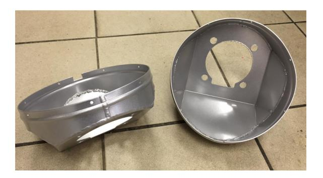
This means your old headlight bowls that are part of your wings need cutting out. Working back from the leading edge, we recommend about the width of a roll of masking tape 1", to make the cut. Make sure to protect your paintworks from the sparks of a cutting disk. Make sure you don't cut too much off! You need to retain the headlight bezel tab as a minimum width for reference. See later pictures.
