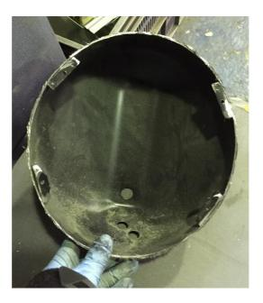
5. Test fit the new headlight bowls, they should be a very tight fit. It is not unusual to have to slit the remaining part of the headlight bowls, to allow it to accept the new bowls.
