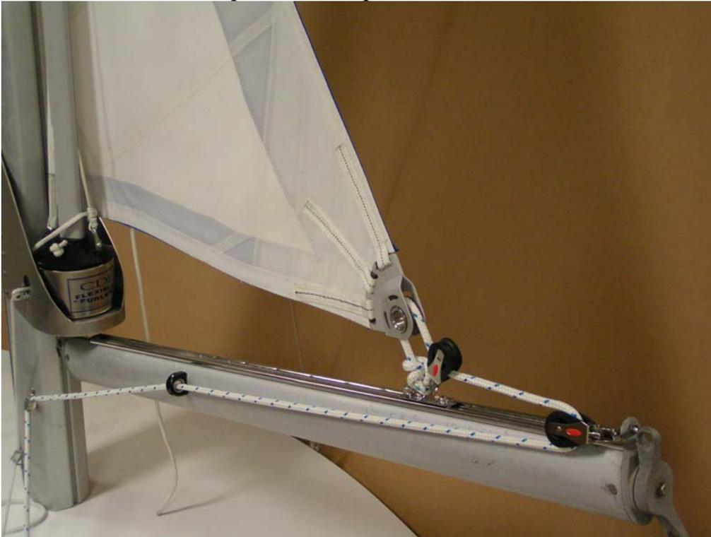
To unfurl or unreef the sail, ease the reefing line, move the reefing car to the end of the boom, and trim in the outhaul line. Always keep some tension on the reefing line to insure a smooth wrap of the reefing line on the drum.
