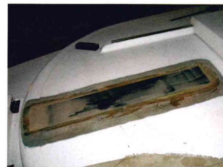
The cabintop mast step on Nathan's Mariner was collapsing, upper left, due to a rotten plywood deck core beneath it, upper center. He cut out the plywood, ground the area clean, and replaced it with carbon-fiber G10 material, upper right. After epoxying the G10 in place, above left, he fiberglassed over it, above center, then faired and painted it. With the mast step back in place, above right, it was as good as new, but stiffer.
