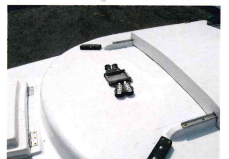
The cabintop mast step on Nathan's Mariner was collapsing, upper left, due to a rotten plywood deck core beneath it, upper center. He cut out the plywood, ground the area clean, and replaced it with carbon-fiber G10 material, upper right. After epoxying the G10 in place, above left, he fiberglassed over it, above center, then faired and painted it. With the mast step back in place, above right, it was as good as new, but stiffer.
