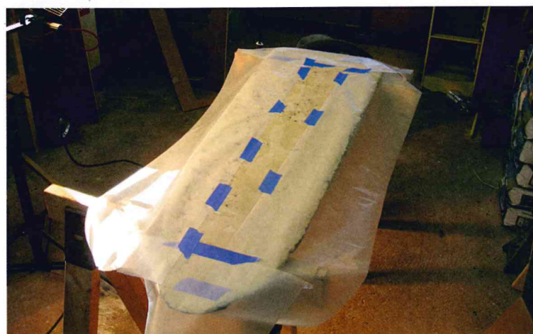
Nathan had a metalworking shop sandblast the centerboard. He then coated it with POR-15 rust-preventive paint and epoxy barrier coats and faired it, using wax paper to wrap and form fairing compound around the edges, at left. Two coats of bottom paint, at right, finished the job.
