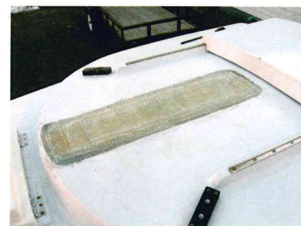
The cabintop mast step on Nathan's Mariner was collapsing, upper left, due to a rotten plywood deck core beneath it, upper center. He cut out the plywood, ground the area clean, and replaced it with carbon-fiber G10 material, upper right. After epoxying the G10 in place, above left, he fiberglassed over it, above center, then faired and painted it. With the mast step back in place, above right, it was as good as new, but stiffer.
