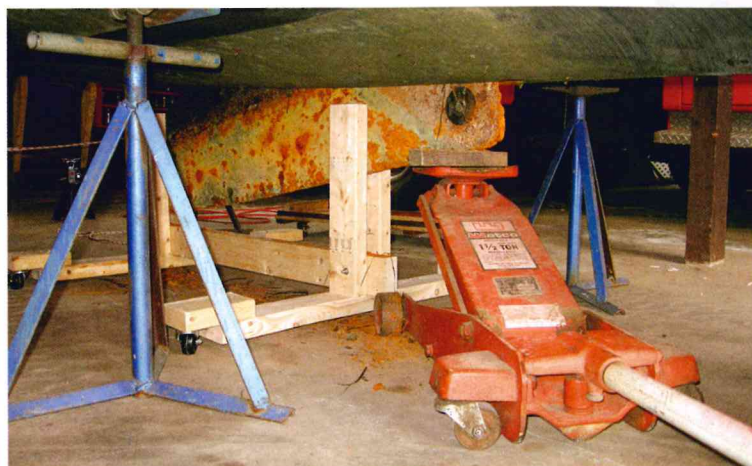
The 165-pound centerboard was covered in rust and presented a challenge. However, Nathan's ingenuity in building a trolley on casters, and muscle in the form of a floor jack, at left, enabled him to extract it and move it around for sandblasting and painting, at right.
