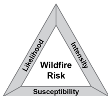
Figure 7. Illustration of risk as the combined influence of the likelihood, intensity, and susceptibility of values to a hazard. Risk is highest when each component is maximized. This triangle has been used to illustrate wildfire risk in a similar format to the fire triangle which illustrates the “ingredients” required for combustion. In this wildfire risk assessment, the spatial interaction of wildfire likelihood, wildfire intensity, and susceptibility of VRAs were evaluated and combined to estimate the expected change in values following wildfire throughout the study area.
