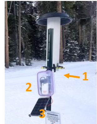
Above: A set up RFID feeder with antennas in the perch (1), a circuit board (2), and a power source (3).
