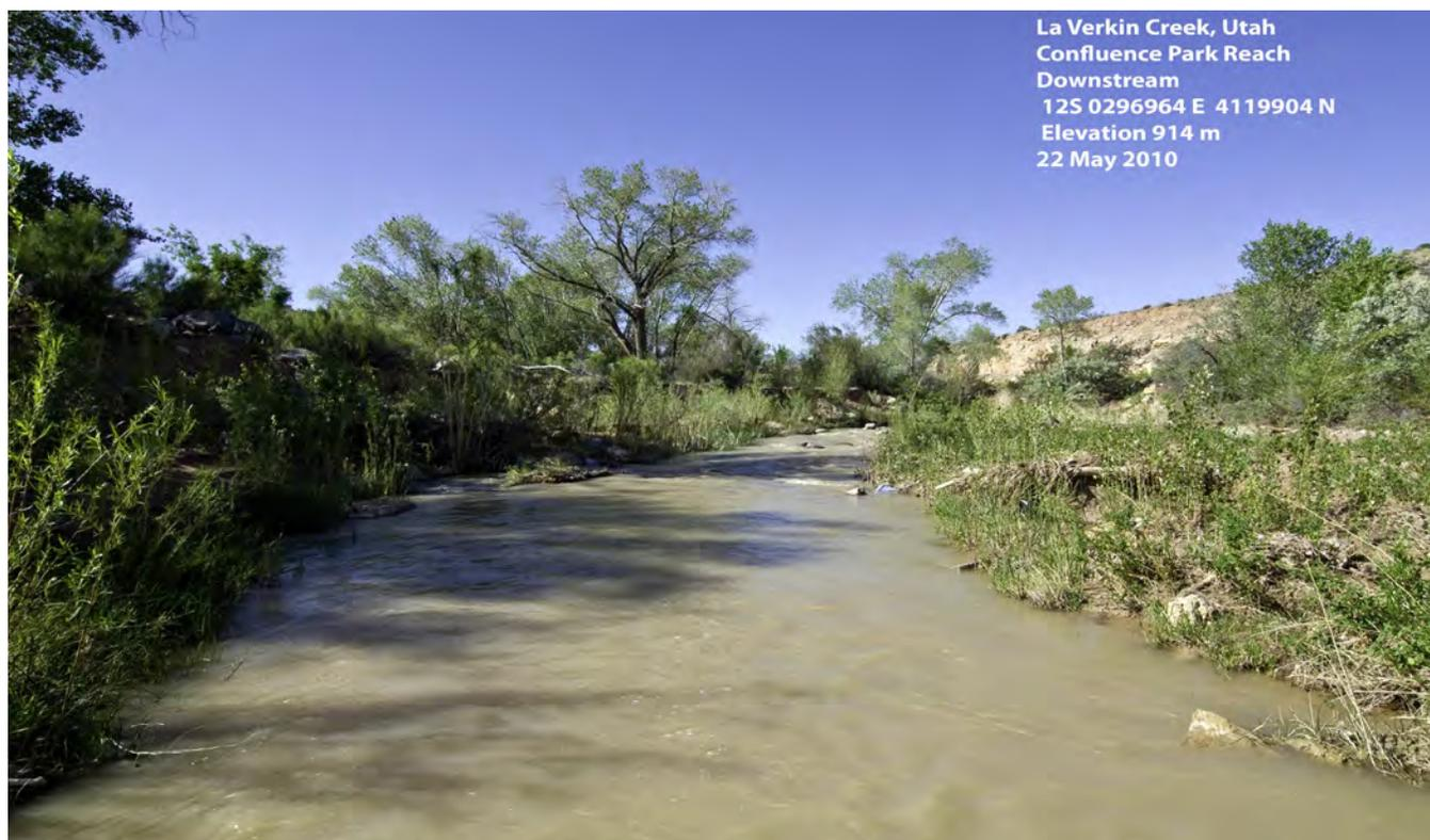
**Figure 3:** Reference photo at the downstream end of a survey reach, looking upstream. Note that the necessary information has been added to the photograph.
