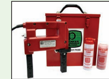
DA-400 Shown With "A" Kit items. Kit items are available with dry powder and Wet Fluorescent inspection mediums. Including Black Light and Steel Carrying Case.
