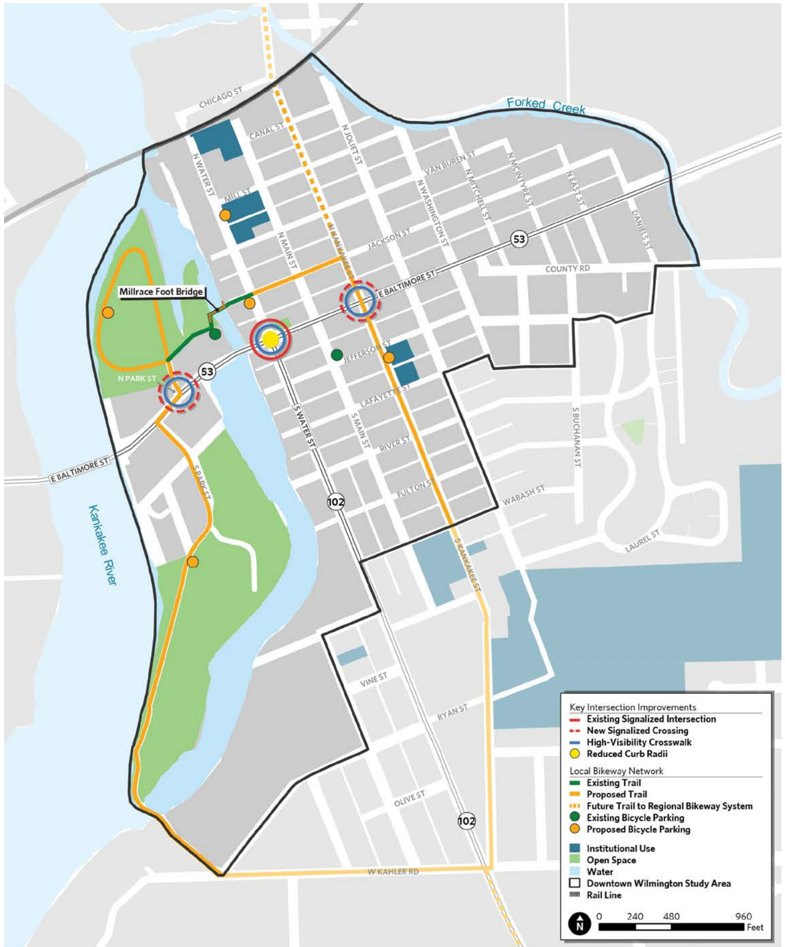
Figure 6.3 Pedestrian and Bicycle Network Improvements
