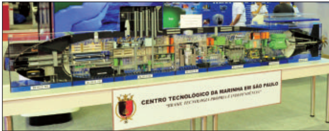
Figure 4. Mock-up of the first Brazilian SSN
