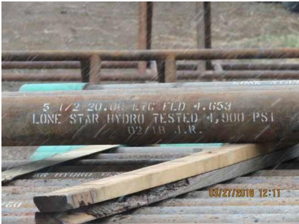
Green Well 5.5 in API drop pipe.
