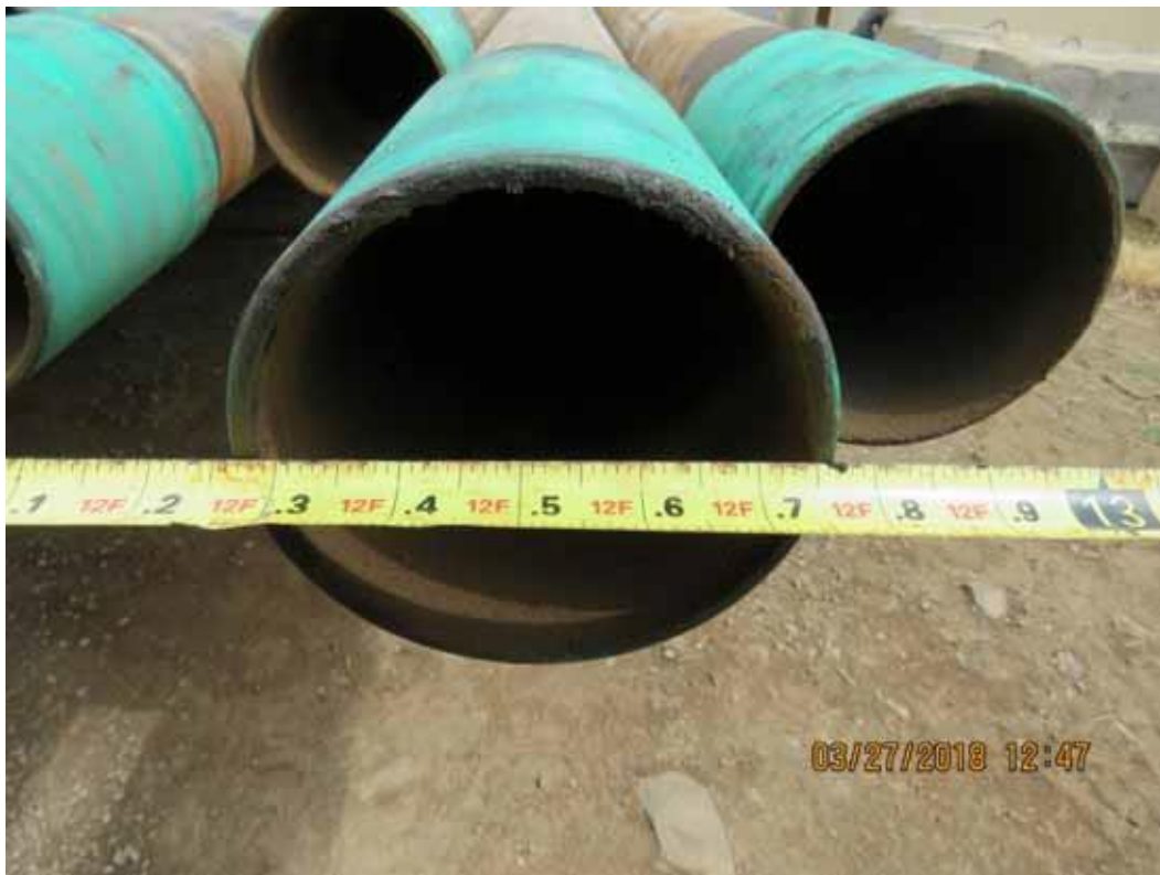
Green Well 5.5 in API drop pipe.
