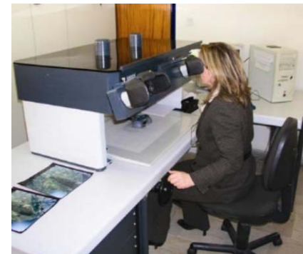
Top: Stereo pair diagram Bottom: Stereo compiler working on a hard copy stereoplotter
