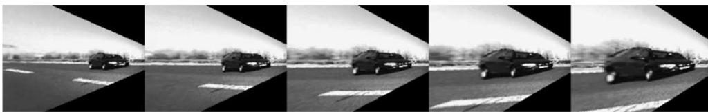
Fig. 17. Consequence of calibration errors on the remapped image. From left to right calibration error of  $-20$ ,  $-10$ ,  $0$ ,  $+10$  and  $+20\%$ .
