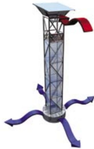
Shower tower air flow diagram
