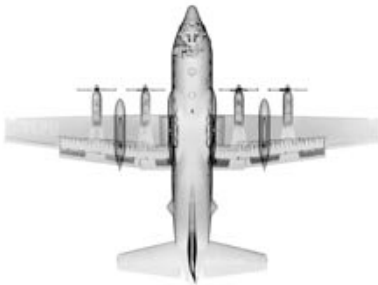
C-130 Hercules transport aircraft scanned in 30 min with no post processing except for visualization.
