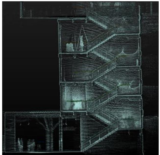
*A five story staircase showing many details of the structure. Traditionally stairs are extremely difficult to map since they are narrow and confining and there is a turn at every landing.*
