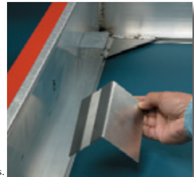
Permanently attach brackets and stiffeners.
