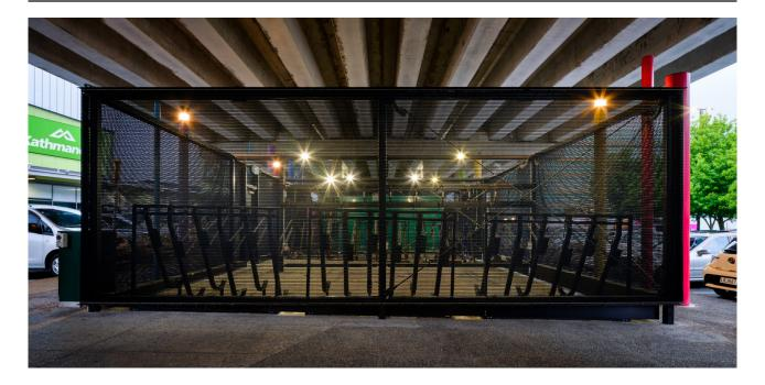
**Kaynemaile**\* is perfect for equipment and enclosure screening - it is extremely lightweight and has great airflow characteristics as well as superior aesthetics compared to traditional screening materials such as louvres or perforated panels.
