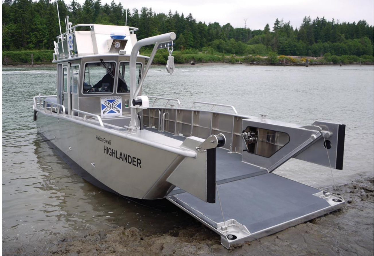
HAIDA GWAII HIGHLANDER, a 30-ft William E. Munson-built (Edmunds WA) landing craft, is the backbone of Danny Robertson's Highlander Marine Services business venture. The bow loading ramp is a necessity for serving remote areas on the islands of Haida Gwaii.
