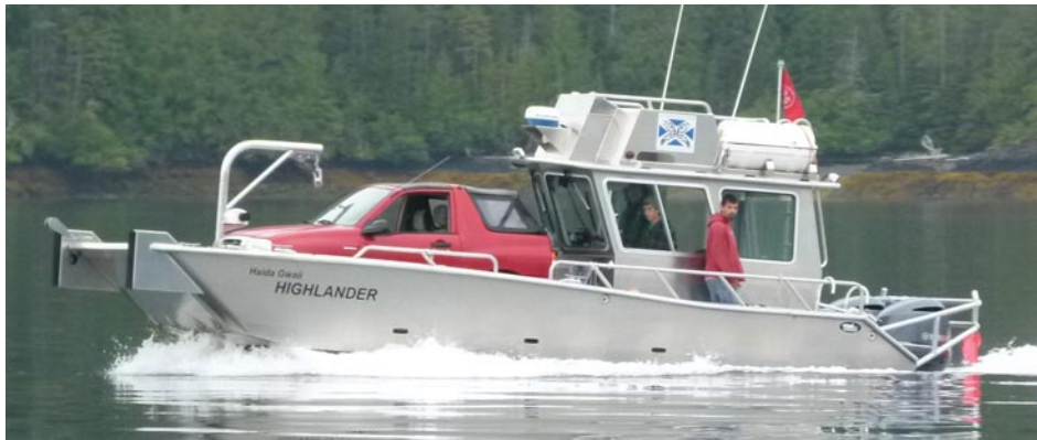
HAIDA GWAI HIGHLANDER underway with a load on. The boat tops out at 40 knots WOT and cruises at 25 knots (both speeds unloaded). Dual 250 hp Yamaha outboards give a reassuring 'get home' capability for remote operations.
