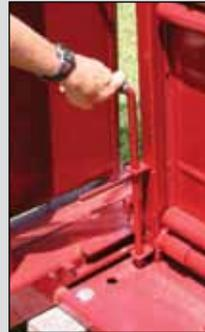
b. Top Width: Using squeeze release mechanism, release squeeze and pull up or down on large squeeze handle to get desired top width. It should be fairly wide when catching and then squeeze applied after animal is caught.
