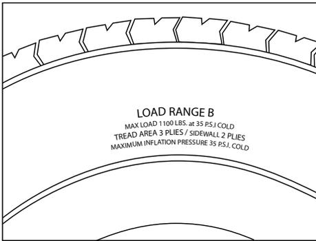
**Figure 2:** Tire Pressure, Load Range & Maximum Load
