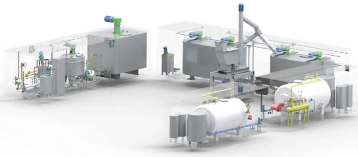
FIGURE 1: GENERAL LAYOUT WITH CRUSHING AND BOILER MODULES
