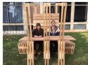
Built in Spring 2016, the picnic table contains a lightweight 100W panel that tracks the sun while simultaneously shading the area for laptop work. In addition, there is a system for battery storage, charge controlling, and data streaming and web interactivity. [[sustain.princeton.edu](http://sustain.princeton.edu)]
