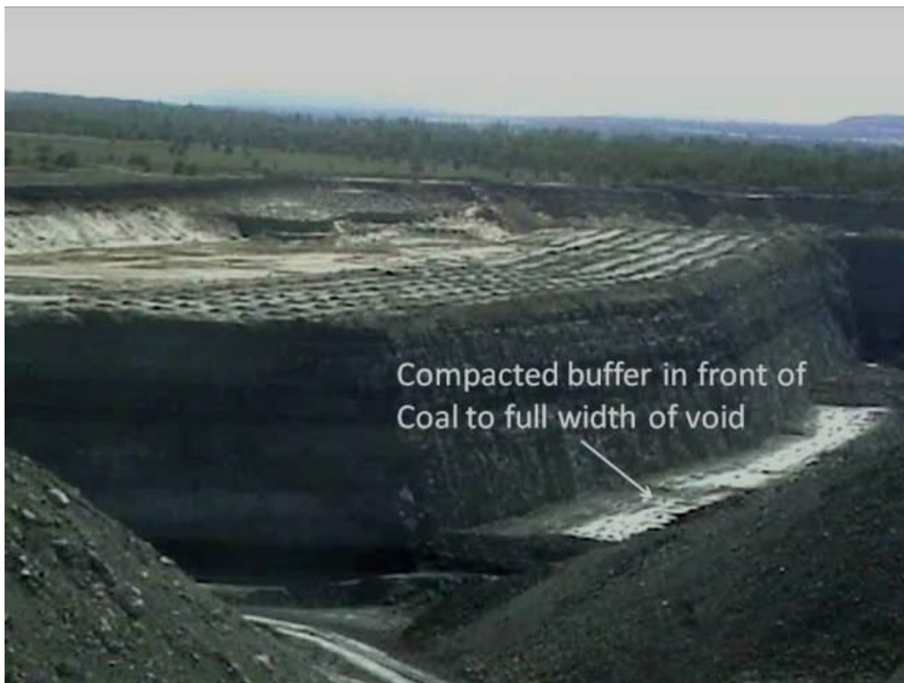
FIG 8 - Throw blast with a baby deck and a large buffer which resulted in significant coal damage and loss
