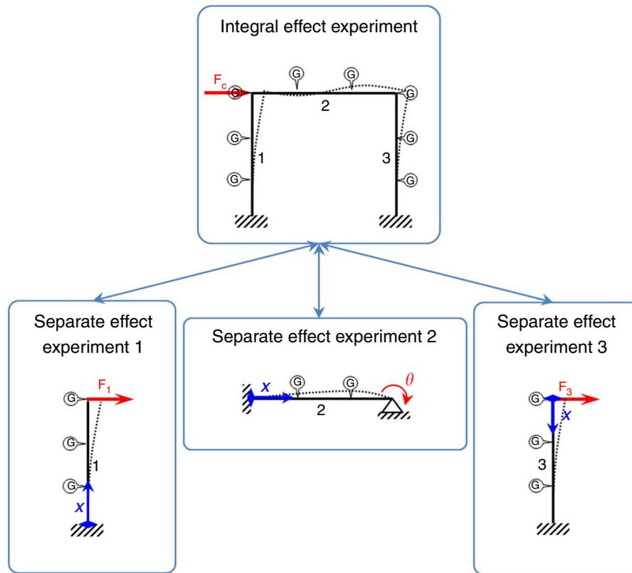
**Figure 5.** Location of the gauges in the portal frame and constituents used to acquire integral-effect and separate-effect experimental data
