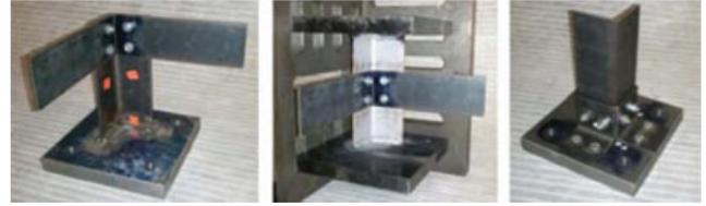
Fig. 13. Connection test specimens: top connection (left), middle connection (middle), and base connection (right).
