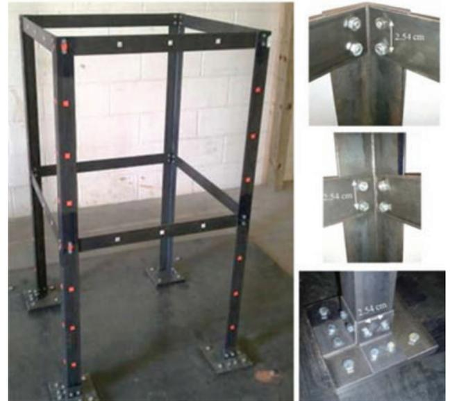
**Fig. 4.** Frame structure built in the laboratory (left) and frame connections (right): top connection (top), middle connection (middle), base connection (bottom).
