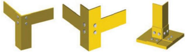
**Fig. 11.** FE connection models: top connection (left), middle connection (middle), and base connection (right).
