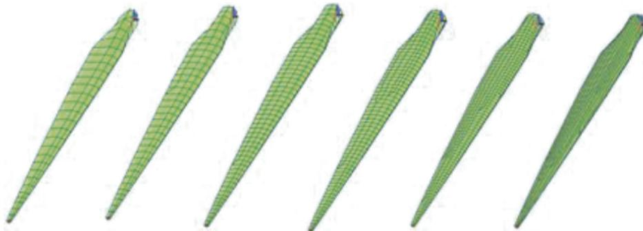
Figure 6: Six representative meshes in ANSYS (coarsest mesh with 62 elements and finest mesh with 10,663 elements).
