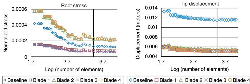
Figure 7: Mesh convergence of the root stress (Left) and tip displacement (Right).
