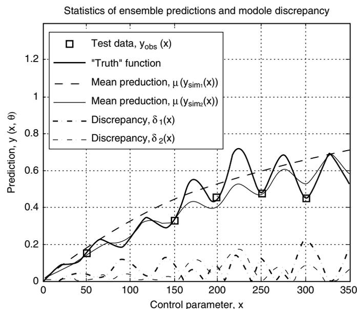
Figure 2: Comparison of Mean Predictions and Discrepancies ( $\delta y_1(x)$  is equal to 8.9% of the mean "truth",  $\delta y_2(x)$ , is 4.6% of the mean "truth").
