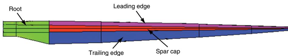
Figure 5: ANSYS model showing different sections of the blade.
