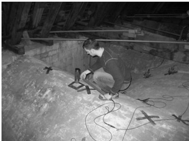
**Fig. 12: The hammer operator hits the predefined excitation points with the sledge hammer while trying to maintain balance on the vaults**
