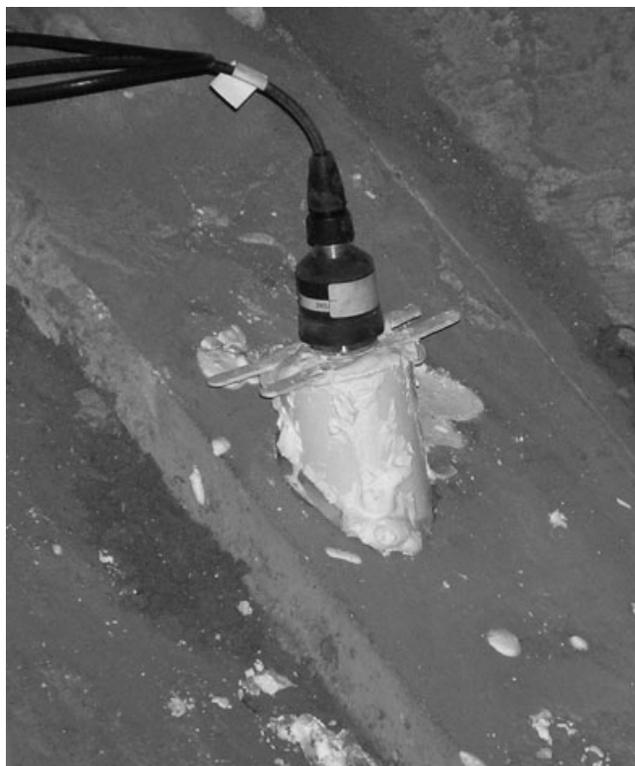
**Fig. 8: Aligning the axis of the sensors vertical on curved surfaces is a difficult task. In our studies, we exploited candles, modeling clay, plaster platforms, and adjustable mounting cases**
