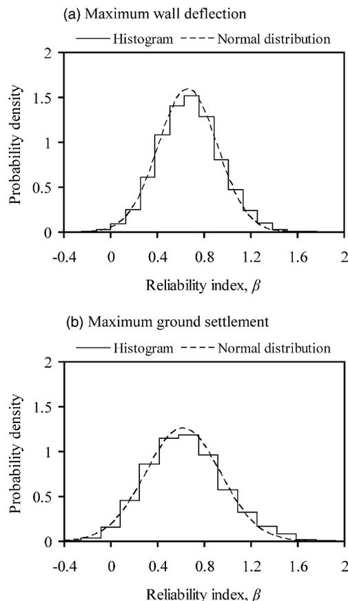
**Fig. 9.** Distribution of the reliability indices computed with the specified limiting: (a) wall deflection; (b) ground settlement (at the final excavation stage)
