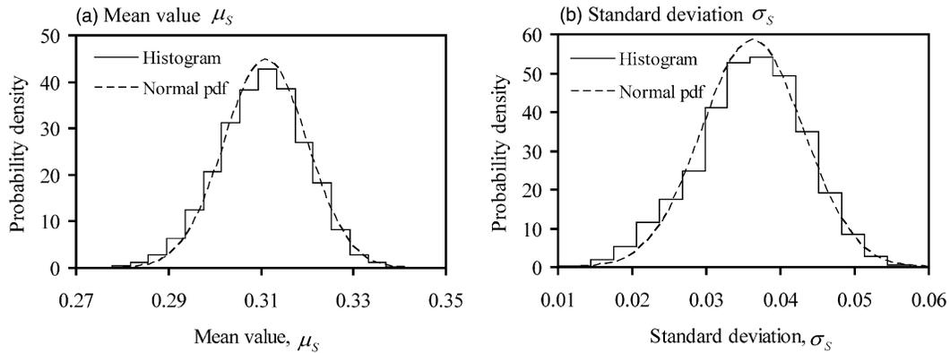
**Fig. 7.** Probability distribution of the mean value and SD of  $s_u/\sigma'_v$
