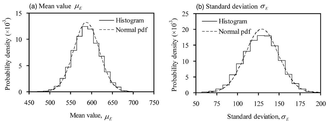
**Fig. 8.** Probability distribution of the mean value and SD of  $E_i/\sigma'_v$
