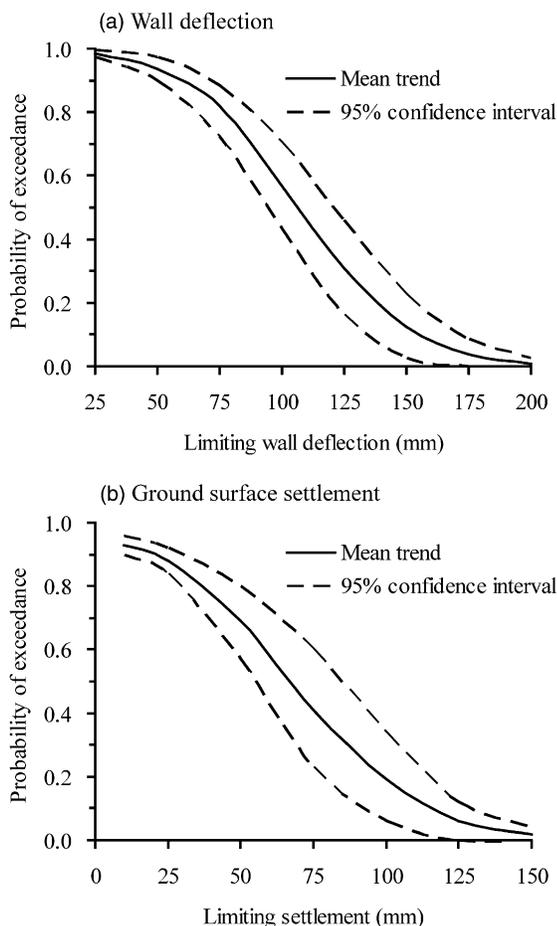
**Fig. 10.** Confidence intervals for probability of exceedance in the TNEC excavation computed with various levels of limiting wall deflection and ground-surface settlement
