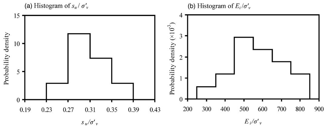
Fig. 3. Probability distribution of the small-strain triaxial test results listed in Table 2
