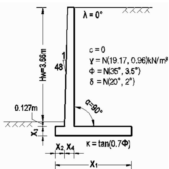
FIG 3. Illustration of the example retaining wall
