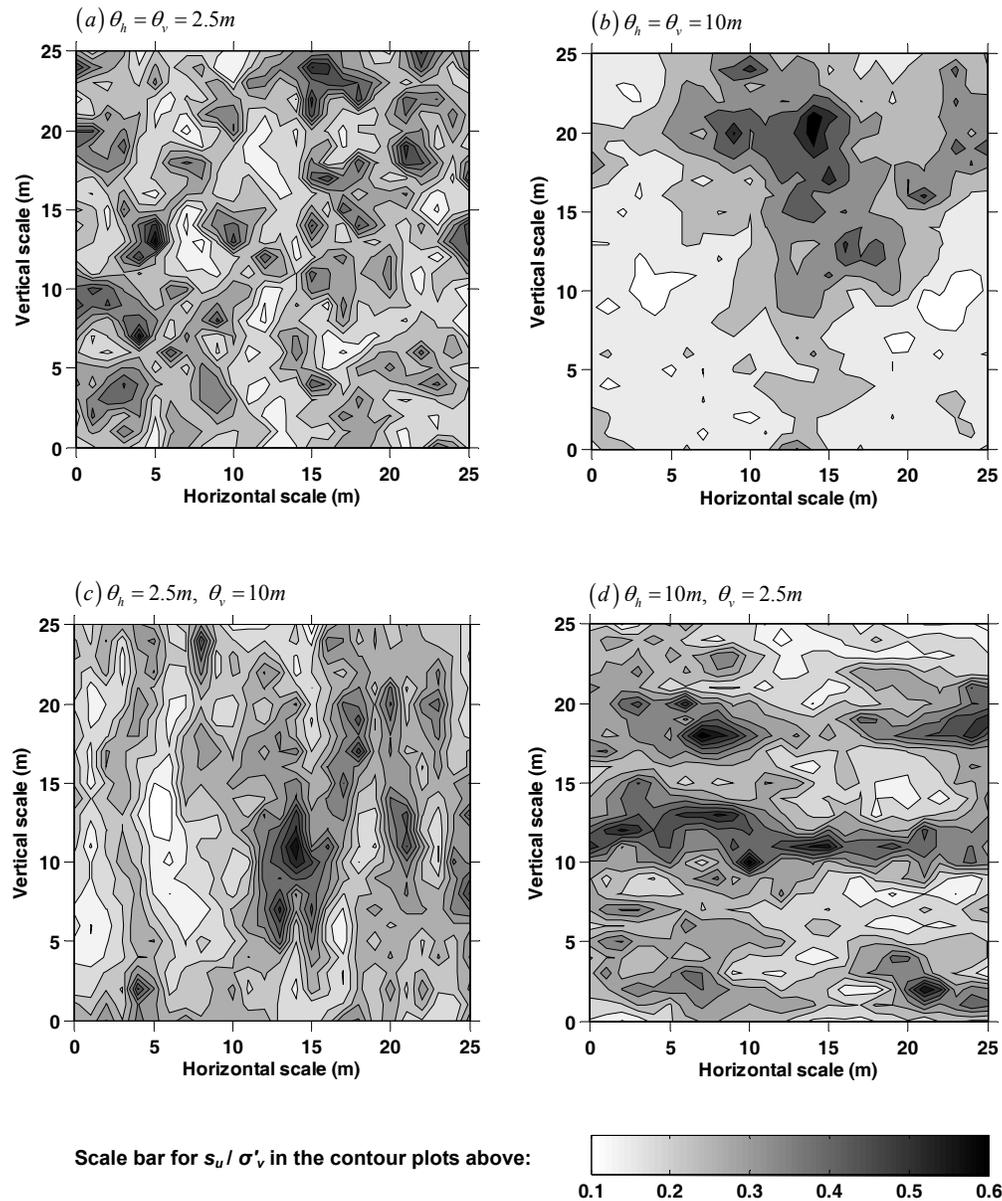
**Figure 2. Influence of scale of fluctuation on the 2-D random field modeling of  $s_u/\sigma'_v$  at given mean of 0.3 and COV of 0.3.**
