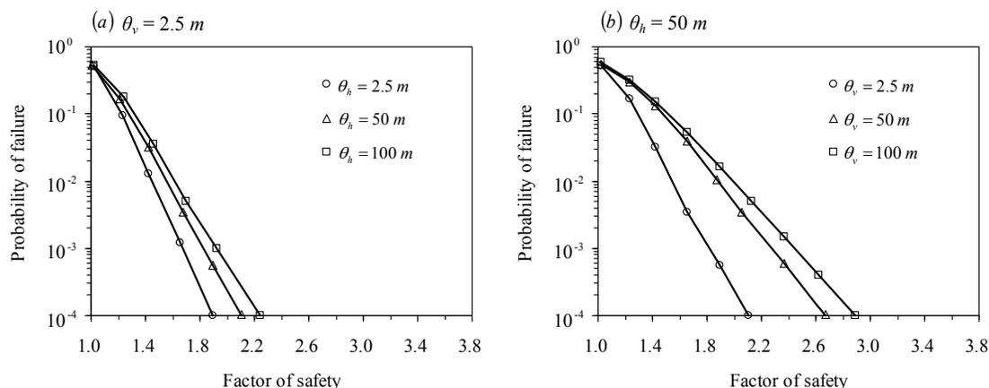
**Figure 4. Effect of 2-D spatial variability on the relationship target failure probability and safety factor.**
