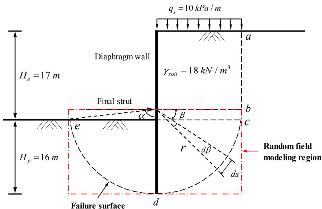
**Figure 1. Geometry of slip circle method and 2-dimensional random field modeling for basal-heave stability (modified from Luo et al. 2012).**
