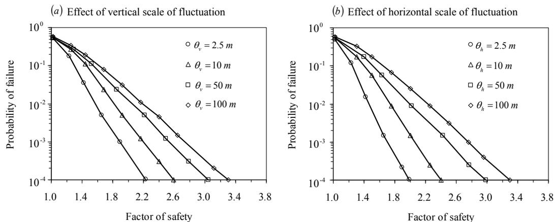
**Figure 3. Effect of 1-D spatial variability on the relationship between target failure probability and safety factor.**
