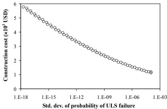
**Fig. 10** Converged Pareto Front for shallow foundation design obtained by NSGA-II based on two-objective (cost and robustness)
