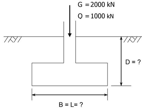
**Fig. 1 A square shallow foundation design example**
