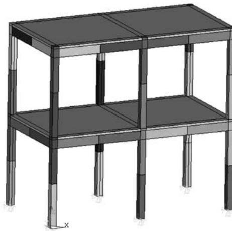
Figure 7. Schematic of different degradation locations.
