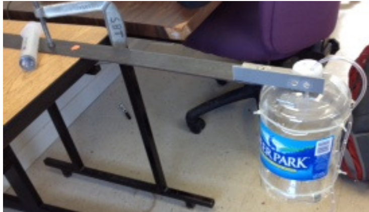
Figure 1: The cantilever beam with mass loading.
