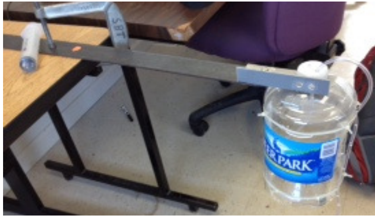
Figure 1: The cantilever beam with mass loading.
