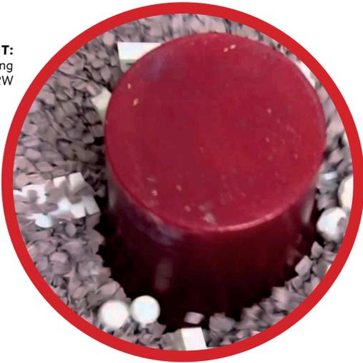
“With vibro-finishing there’s a limit to how delicate a part can be,” says Rowley. “There are also issues about details and undercuts on parts, the chips aren’t always small enough to get into certain spaces so you get a nice finish on the open surfaces but the bits where the chips can’t get in remain unpolished.”
