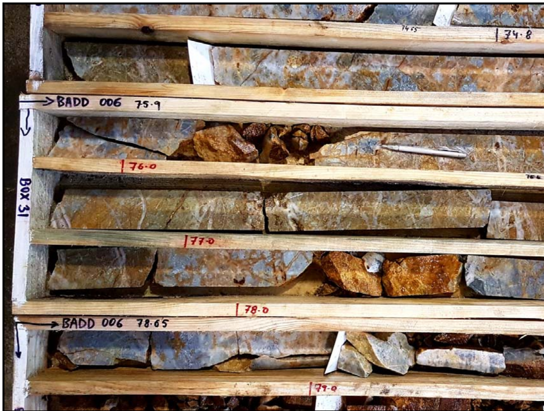
Diamond drill core of BADD006 core showing the mineralised quartz-stockwork. The position of the visible gold is indicated by the pointer.
